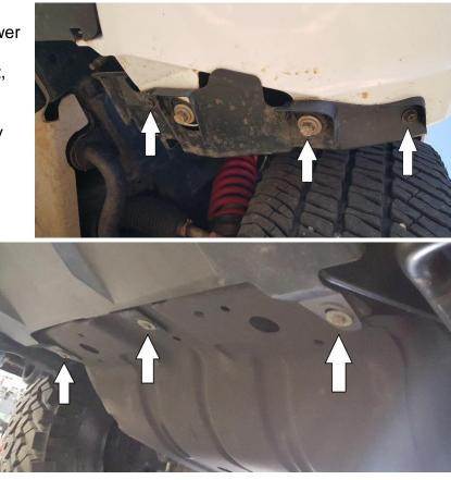
2. Remove the (8) 14mm nuts holding the bumper on. Remove the bumper.
