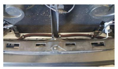
**16.** Plug your fog lights and parking sensors back in. Reinstall the 2 outer plastic covers for the bumper with the (4) 10mm, (1) 12mm, and 1 plastic clip hardware. Reinstall the (3) 10mm bolts holding the lower bumper plastic to the skid plate.
