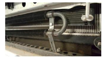
**9. 2010-2013 Models only.** Mark the inside edge of the lower sheet metal section of the factory bumper on both sides. Cut the sheet metal and remove the center section. Clean up all sharp edges on remaining sheet metal.
