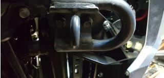
\*Note: If you have a TRD Pro or TRD Pro skid plate you need to add the provided spacers between the lower supports and winch mount using the included longer bolts.
