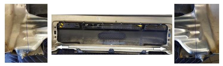
**10. 2014+ Models only.** Place the bumper skin on the mount and mark where the winch cables may come in contact with the factory bumper. Trim the sheet metal on bumper to clear as shown.
